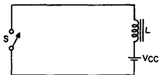
Fig. 85—Simplest form of deflection circuit.
